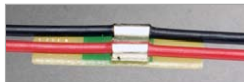
Figure 3: Wires Properly Terminated by the Press
